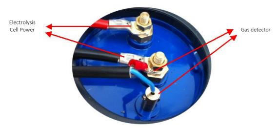
Fig 5 - Electrolysis Cell Connection Terminals
