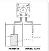
Connect the pump to the timer (or Power Socket 240V AC) The pump will discharge 0,08 cL every 2 seconds.
