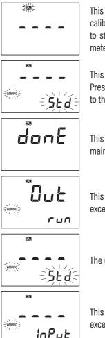
This screen appears each time the meter enters pump or pH calibration mode by pressing the **CAL** button. The meter is ready to start pump calibration by pressing the **PUMP** button. The meter returns to the main screen by pressing the **CAL** button.
