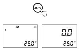
Gently absorb the ZERO water standard with a soft tissue. Use care not to scratch the prism surface. Wipe off the surface completely. The instrument is ready for sample measurement. *Note:* If instrument is turned off the calibration will not be lost.
