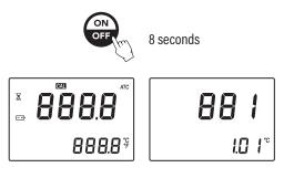
While continuing to hold the ON/OFF key, press the ZERO key. The temperature unit will change from °C to °F or vice versa.
