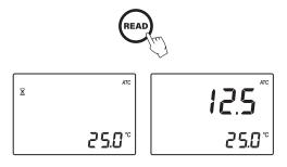
**Note:** The ATC tag blinks and automatic temperature compensation is disabled if the temperature exceeds the 10-40  $^{\circ}C$  / 50-104  $^{\circ}F$  range.
